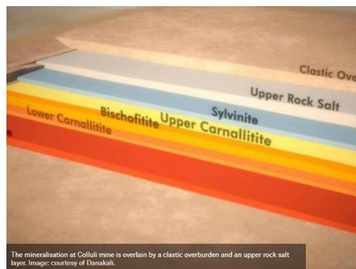
Figure 1.16 Colluli potash mineralization
