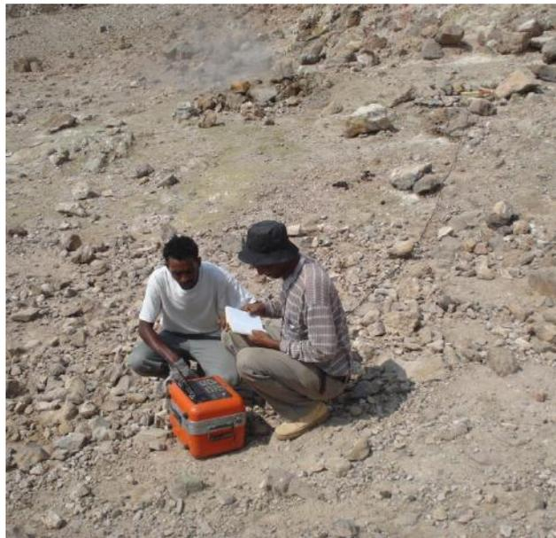
**Figure 8.** TEM survey on Mount Alid. Note the steam vent in the back (photo: Andemariam Teklesenbet).
