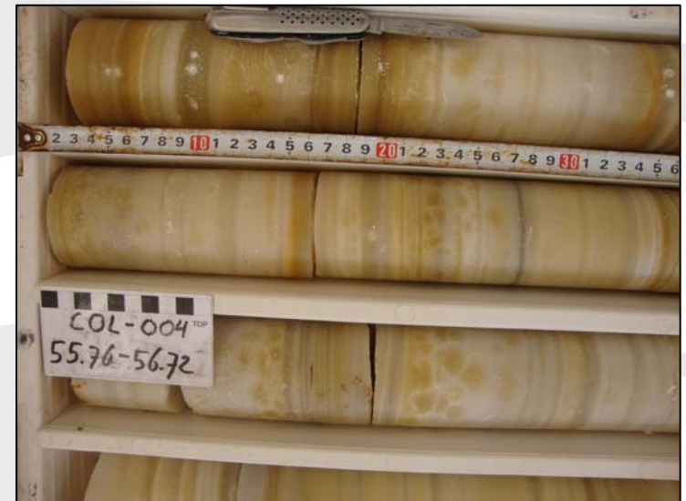
COL-004 drill core showing high grade carnallite and kainitite mineralisation.
